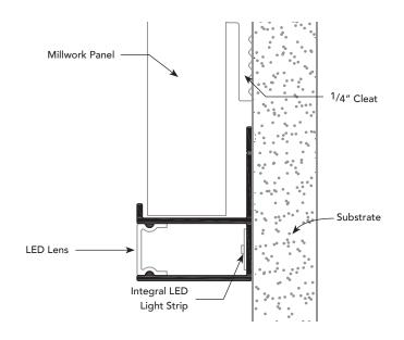
Fry Reglet Lighted Millwork Channel F with exposed return key installs with 1/2", 3/4" or 1" millwork panels, features an exposed return key to cover cut edges of millwork panels, and provides a continuous band of light horizontally or vertically. Frosted lens included.
